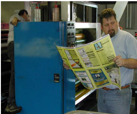
Brad and Jim checking a directory for quality and watching signatures being jogged off the end of the press
